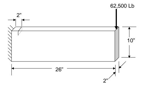
Material: Titanium 6AL-4V E = 16 x  $10^6$  PSI K<sub>IC</sub> = 60.0 KSI  $\sqrt{in.}$ Sy = 130.0 KSI Crack Depth = 0.3 in.
