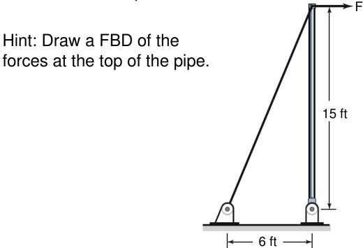
If a horizontal load (F) of 3000 Lb is applied, what is the factor of safety against buckling?
