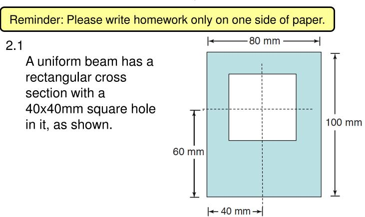
If the beam is to be loaded by a moment applied as shown below, calculate the location of the neutral axis, and then the Area Moment of Inertia needed to determine the bending stress on the top and bottom faces of the beam.
