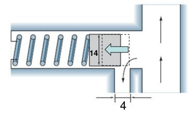
A pressure relief valve, shown here, has a piston diameter of 14 mm and a slit length of 4 mm. The spring has mean coil diameter D = 12 mm and wire diameter d = 2.5 mm. The valve should open [at the dashed position] at 1.5 bar (0.15 MPa) pressure and be totally open [clearing the slit] at 4.5 bar (0.45 MPa) pressure, at which time the spring is fully compressed. The shear modulus for the spring material G = 80 GPa. The spring ends are squared and ground.
