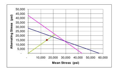
The Repair Wrench sees a bending moment of 85 FtLb, resulting in a bending stress of 42.6 KSI in alternate directions as the bolts are first removed, then replaced. So this is fully reversing. The 1000 cycle stress level, SL = 0.9 Sut = 51.3 KSI. Se is as above. The curve parameters are  $a = SL^2/Se = 92.34 KSI$ , and b = -1/3 Log10(SL/Se) = -0.08509. The life at 42.6 KSI = (AltStress/a)^(1/b) = 8990 cycles.
