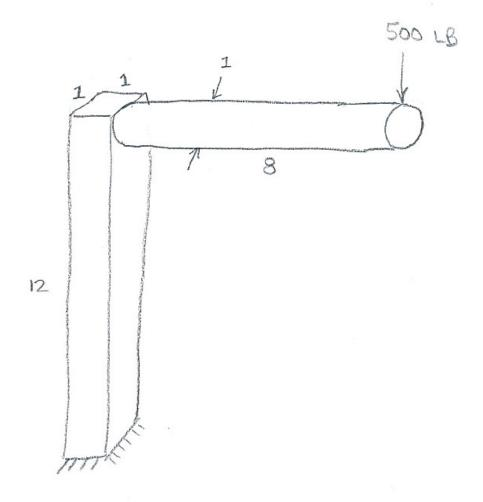
Material is steel with a Modulus of Elasticity of 30 million psi. Dimensions are in inches.
