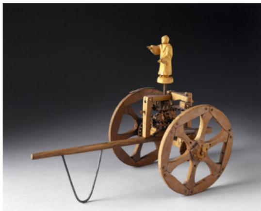
The South-Pointing Chariot was a two-wheeled vehicle in ancient China with a moveable pointer that always pointed south, no matter how the chariot turned.
