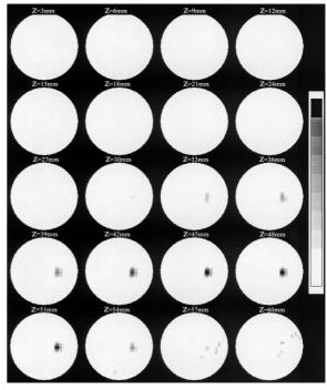
Fig. 4. Images reconstructed from simulated data when the object was located at a distance of 15 mm (z = 45 mm) from the exit plane. The sequence of circles represents images at 3-mm intervals along the cylinder axis. The linear intensity scale spans the range 0–20. The maximum value of  $\Delta \mu_{\alpha}(\mathbf{r})$  is 0.04 mm<sup>-1</sup> and the size of the object is  $3 \times 3 \times 3$  mm<sup>3</sup>.
