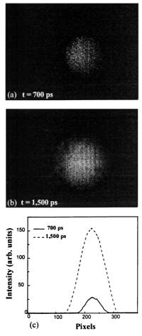
Fig. 2. Experimentally measured 2-D intensity distribution of light transmitted through the scattering medium with the object for a gate position of (a) 700 ps and (b) 1500 ps. (c) The object was located approximately on the axis of the cylindrical cell at a distance of 15 mm from the exit plane.
