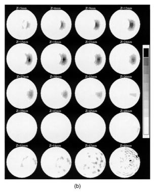
Fig. 6. Images reconstructed from simulated data when the object was located at a distance of (a) 30 mm (z = 30 mm) and (b) 45 mm (z = 15 mm) from the exit plane. The sequence of circles represents images at 3-mm intervals along the cylinder axis.
