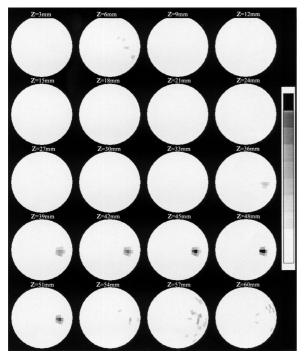
Fig. 7. Images reconstructed from simulated data when the object was located at a distance of 15 mm (z = 45 mm) from the exit plane. Image reconstruction was carried out with data collected using the direct arrangement of both the source and the detector, as well as reversing their positions in the *z* direction.
